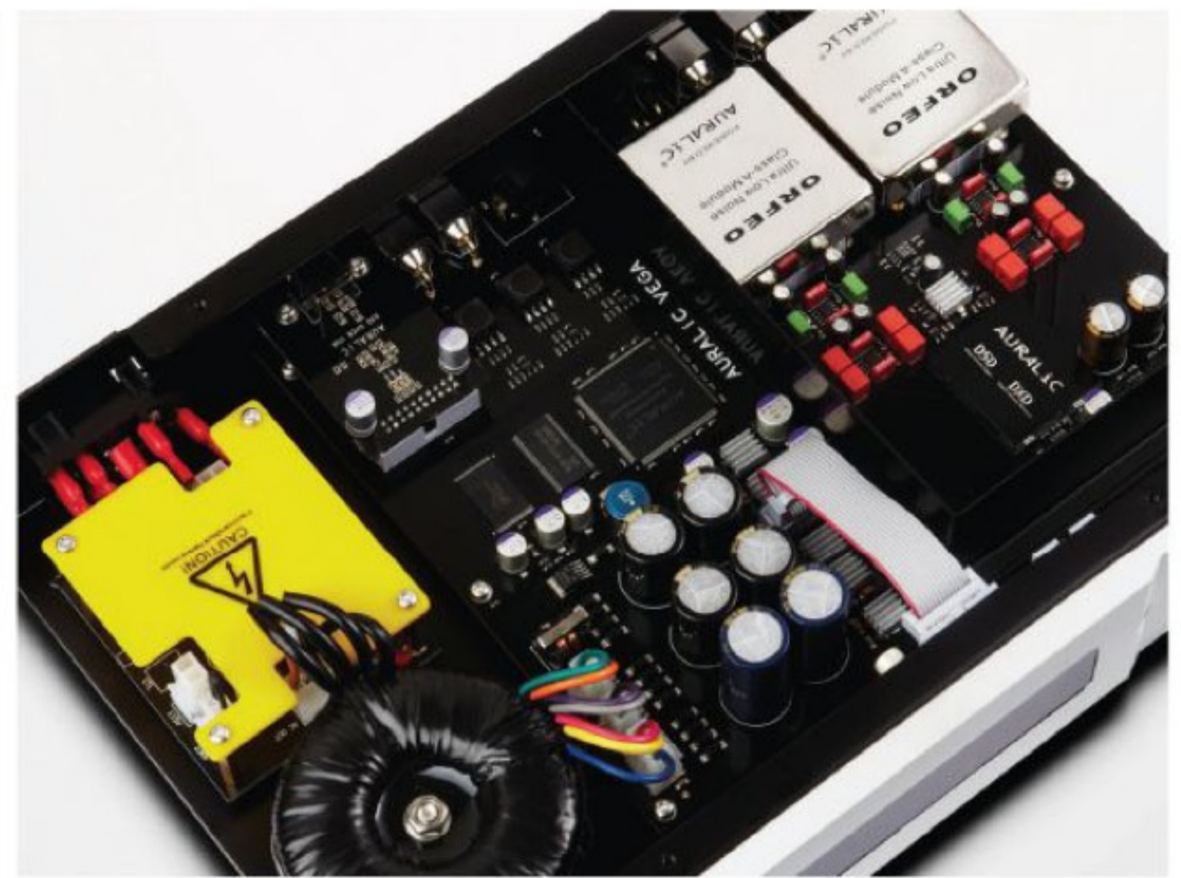
The large, square chip in the center of the PCB is the Sanctuary audio processor.
